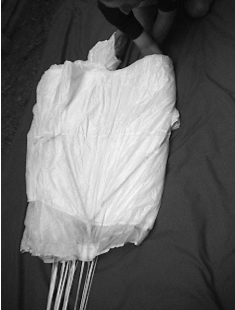
20. Place C lines on top of B lines.
